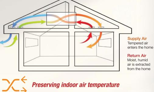
A Heat Recovery System is designed to bring fresh air into your home at a comfortable temperature. These systems recover heat or cooling energy from extracted room air as the heat recovery core transfers the heat from the outgoing air to the incoming air, warming or cooling your home respectively.
