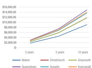
Mechanical ventilation with heat recovery units (MVHR) offer additional energy savings above and beyond that of a typical ventilation system. **Assumptions:** The savings shown here are purely based on potential heating cost savings when reheating air through a 90% efficient MVHR running continuously verses a direct air system to achieve 20°C+ year-round for an air volume based 0.35ACH in a 150m² house with a 2.4m ceiling height using electric heat at 30 cents/kWh.
